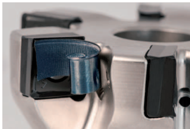
Perfectly adapted chip pockets
