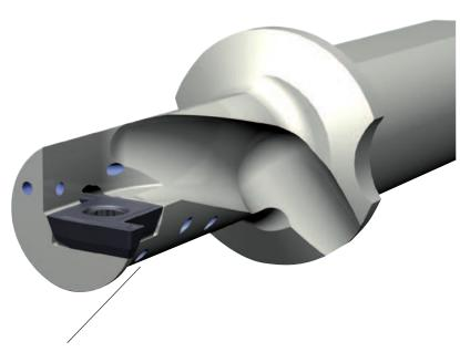
Due to the insert size the diameters 10 mm and 12 mm can be applied only as  $90^{\circ}$  version. For this reason the new tools are provided with a support in the area of the parting and grooving blade in the insert seat to increase stability.
